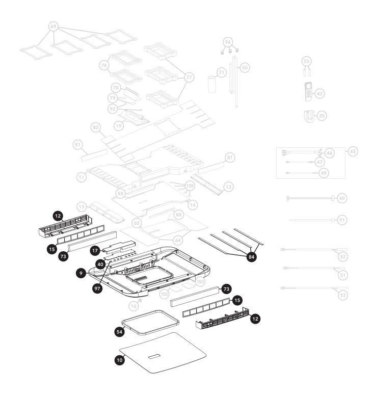
The indoor unit cover is available as a complete spare part under item number 1504930 and consists of the following components: 9, 10, 12, 15, 17, 40, 54, 73, 84, and 97.
