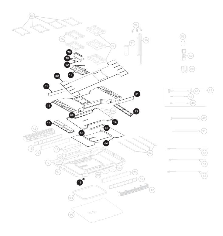
The internal air distributor is available as a complete spare part under item number 1504940 and consists of the following components: 11, 13, 14, 16, 19, 64, 65, 78, 79, 80, 81, 88, and 92.
